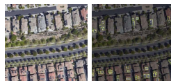
Left: unannotated image with solar panels. Right: annotated image with solar panels using square bounding boxes [3].
